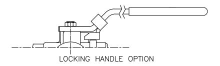
NOTE: LOCKING HANDLE OPTION AVAILABLE LOCKING HANDLE ORIENTATED 180° FROM NON-LOCKING HANDLE. LOCKING HANDLE PART NUMBER DENOTION: BHM-##LL
